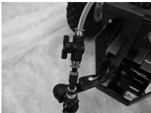
Figure 6 shows the in-line 8mm 2 port bleeding valve that connects the pump outlet to the spray head.
